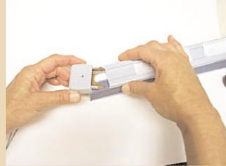
2. Remove cord lock and color cap by pulling out of headrail.
