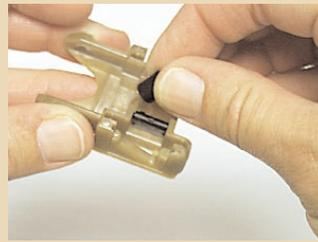
6. Next slide the roller onto the post of the base. There is no top or bottom on the roller.
