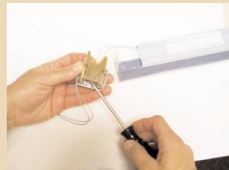
3. Pry off color cap cover to expose cord lock assembly. Pull cord out and away from assembly and discard assembly.
